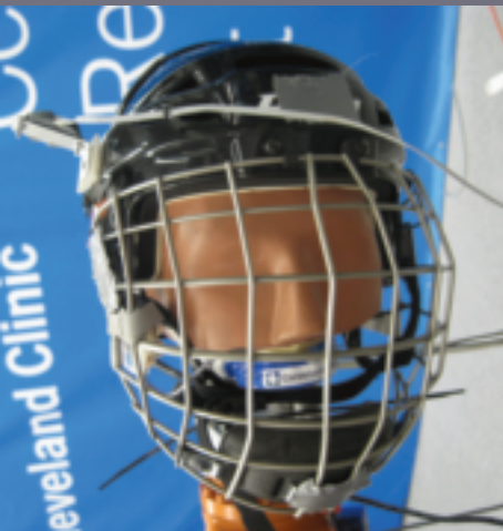
◀ The Intelligent Mouthguard is tested on a crash test dummy headform via a robotic testing arm in the Cleveland Clinic Head, Neck and Spine Research Laboratory.
