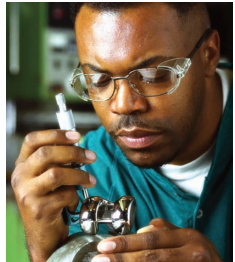
Mr. Curtis Johnson performs a dimensional inspection of a finished Wright knee implant component.
