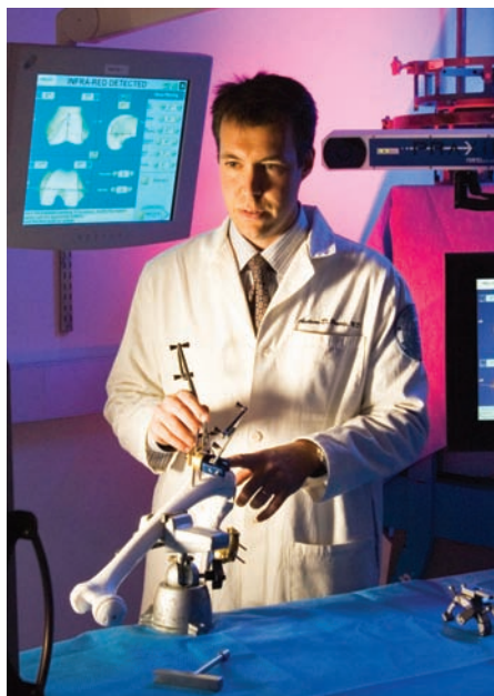
The Computer Assisted Surgery Center at Hospital for Special Surgery aims to develop and validate surgical navigation and medical robotics in orthopaedic surgery. Here, Andrew D. Pearle, M.D. demonstrates the acquisition of reference points by navigated instruments to help plan knee replacement surgery.
